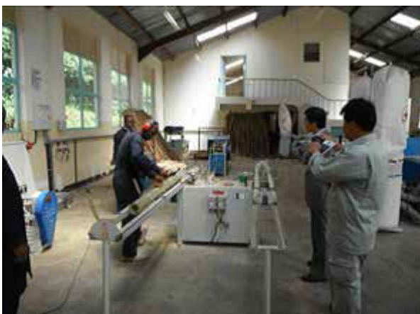
Fig. 4.2: Splitting bamboo culms
