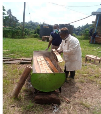
Fig. 4.3: Bamboo culms submerged in preservative
