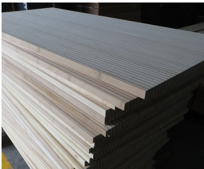
Fig. 4.4: Finished Bamboo boards
