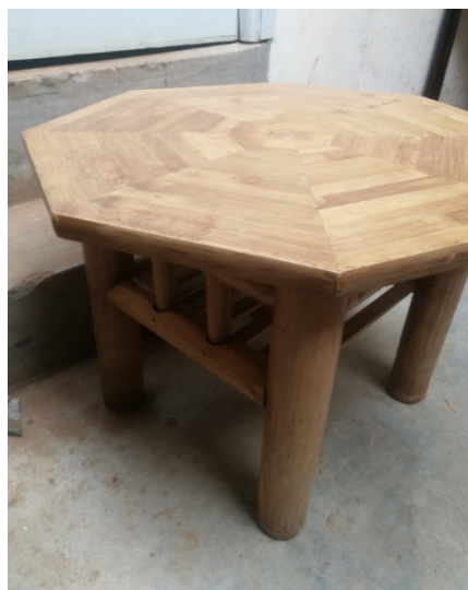
Fig. 4.5: Laminated table top with a unique arrangement of bamboo slats glued together
